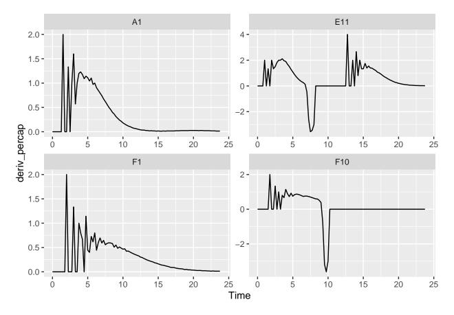
These derivatives are very jumpy. Why? The same limited resolution of the plate reader has an amplified effect on the per-capita derivative when densities are very close to 0. Luckily, calc\_deriv can calculate derives by fitting a linear regression to multiple points, reducing this jumpiness in the derivative.
