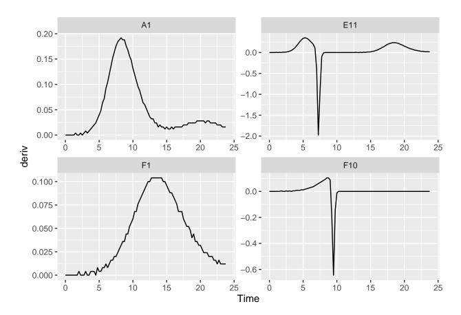
You might notice that these lines aren't super smooth. Why? The plate reader data has a limited resolution, only to the nearest 0.001, causing the derivative to "jump" when the reading increases.
