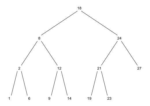
Figure 1: A balanced binary tree with 13 elements.
